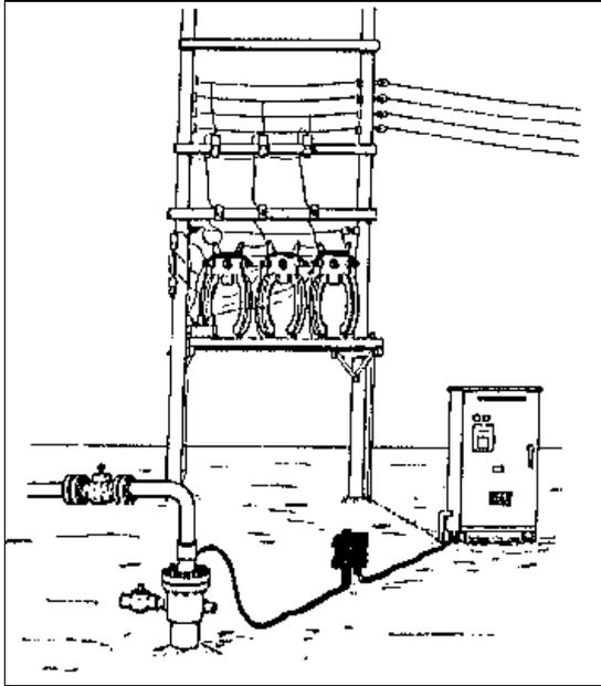
**Figure 2. The surface equipment, including the power line, transformers, control box, meter chart, and wellhead.**
