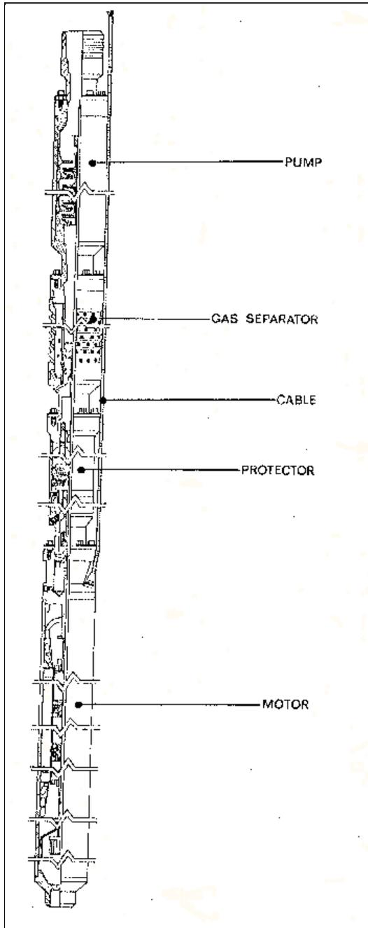
**Figure 1. A motor and pump assembly.**
