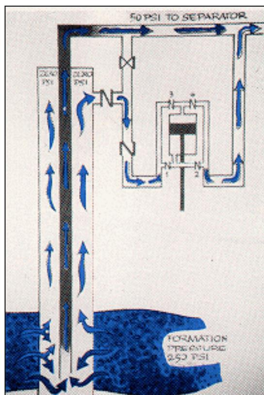
**Figure 2.** Beam gas compressor operation. (courtesy of Permian Production Equipment, Inc.)
